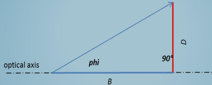
$B$ : distance between a plane and the measurement location.
